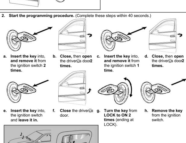
i. The tail and marker lights flash 2 times, the buzzer chirps 2 times and the doors lock and unlock 2 times.\*
