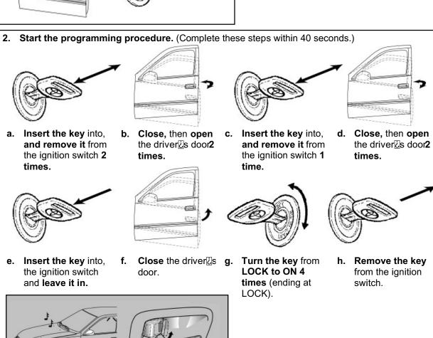
The tail and marker lights flash 4 times, the buzzer chirps 4 times and the doors
